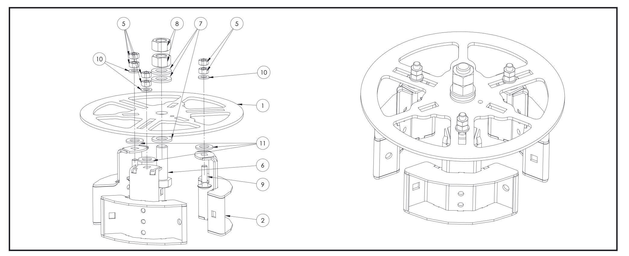
ASSEMBLE MC TOP MOUNTING PLATE TO PIPE CLAMP TOP
