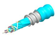
Fiber indoor cable, LazrSPEED® Low Smoke Zero Halogen Riser MPO Trunk, interlocking aluminum armored with low smoke zero halogen riser jacket, Multimode OM4, 16 fiber, Gel-free, Feet jacket marking, Aqua jacket color, B2ca flame rating
