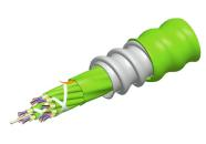
Fiber indoor cable, LazrSPEED® Plenum MPO Trunk, interlocking aluminum armored with plenum jacket, Multimode OM5, 96 fiber multiunit with 8 fiber subunits, Lime-green jacket color, Feet cable marking
