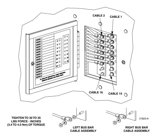
Figure 29. Cable Grounding System - Exterior View
