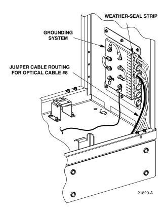
Figure 28. Cable Grounding System - Interior View
