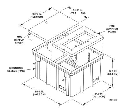
Figure 3. Mounting Sleeve (FMS-FD3J-KIT-A)
