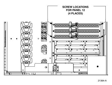
Figure 25. Secure Distribution Panel to Front Side of Swing Frame
