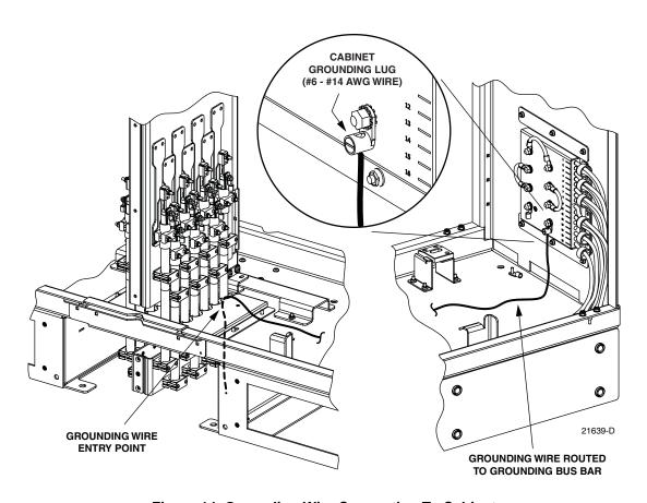
**Figure 14. Grounding Wire Connection To Cabinet**
