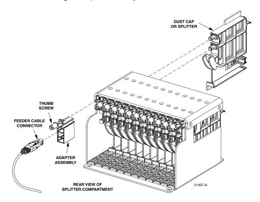
Figure 39. Splitter Compartment Adapter Replacement
