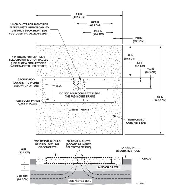
Figure 9. Constructing the Concrete Pad for the 864 Termination FDH 3000 Pedestal-Mount Cabinet
