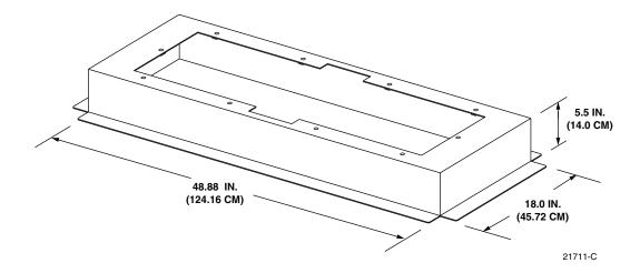
**Figure 8. Pad Mount Frame Dimensions**
