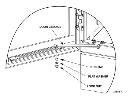
Figure 41. Door Linkage Hardware
