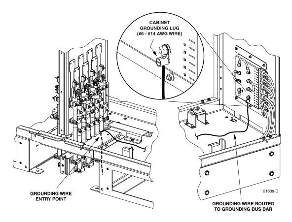
Figure 7. Grounding Wire Connection To Grounding Bus Bar
