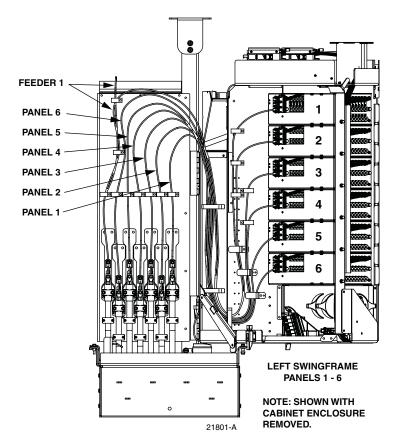
Figure 26. Route and Secure Distribution Cable Subunits - (Panels 1 – 6)
