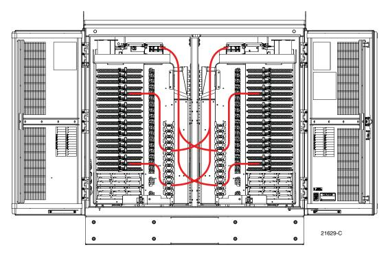
Figure 32. Routing Splitter Output Fibers - Splitter and Distribution Port on Opposite Sides of Cabinet
