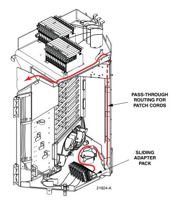
Figure 37. Routing Patch Cord Through Left Swing Frame
