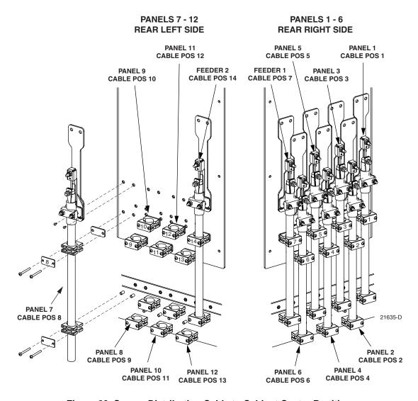
Figure 22. Secure Distribution Cable to Cabinet Center Partition
