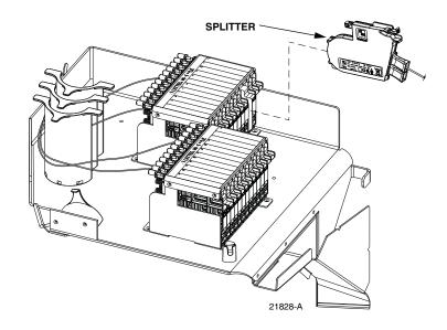
Figure 20. Splitter Installation
