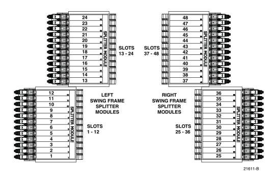
Figure 17. Splitter Compartment Layout - Top View
