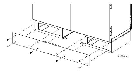
Figure 6. Removing Access Covers From Ground Spacer/Riser
