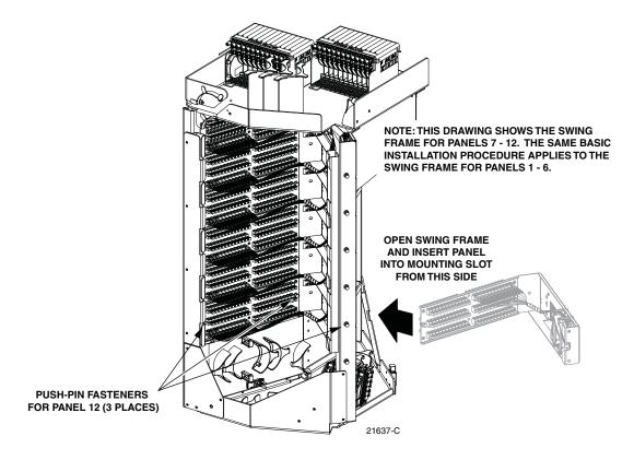
Figure 24. Inserting Distribution Panel into Swing Frame Mounting Slot - Typical
