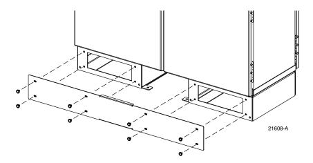
Figure 13. Removing Access Covers From Ground Spacer/Riser
