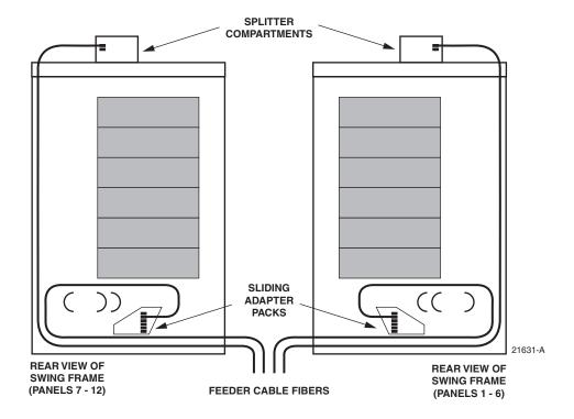
Figure 15. Feeder Cable Typical Configuration
