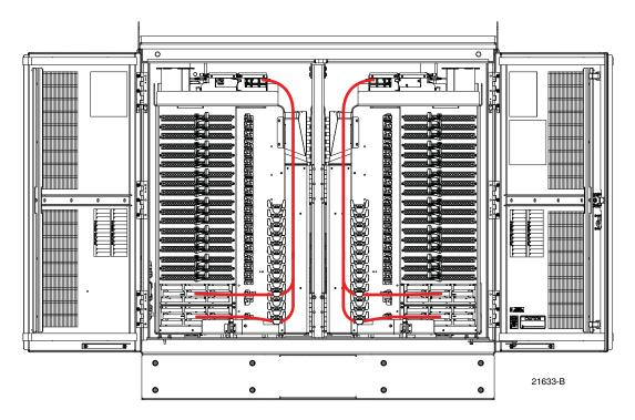
Figure 30. Routing Splitter Output Fibers for Storage
