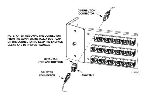
Figure 38. Adapter Removal and Replacement
