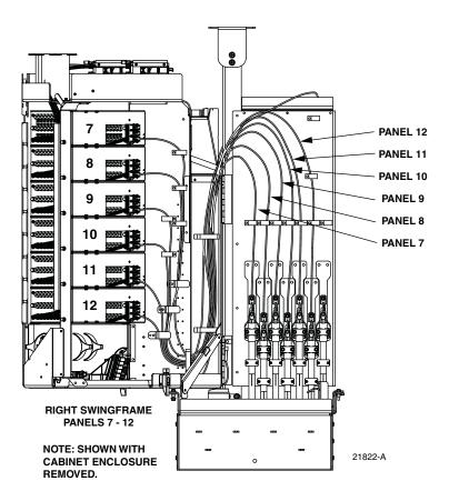
Figure 27. Route and Secure Distribution Cable Subunits - (Panels 7 – 12)
