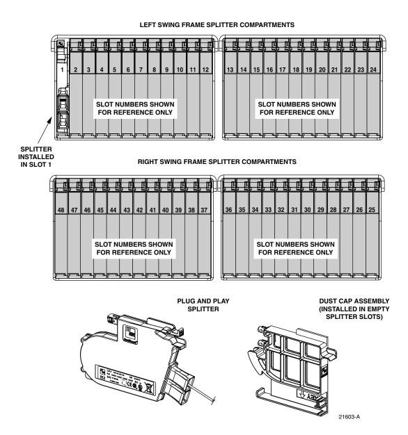
Figure 18. Splitter Compartment Mounting Slot Assignments
