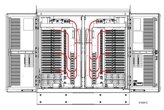
Figure 31. Routing Splitter Output Fibers - Splitter and Distribution Port on Same Side of Cabinet
