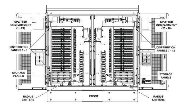
NOTE: THE CABINET IS EQUIPPED WITH A LEFT AND RIGHT SWING FRAME. EACH SWING FRAME ROTATES OUTWARD TOWARD THE FRONT OF THE CABINET. THIS PROVIDES ACCESS TO MOST OF THE COMPONENTS MOUNTED WITHIN THE CABINET.
