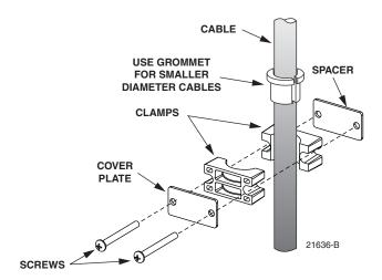
Figure 23. Cable Clamp Assembly
