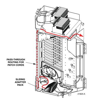
Figure 36. Routing Patch Cord Through Right Swing Frame
