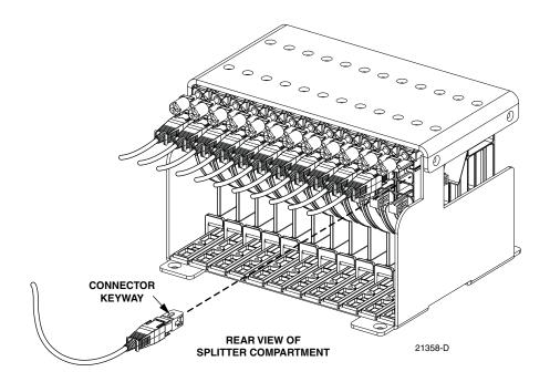
Figure 19. Feeder Cable Connector
