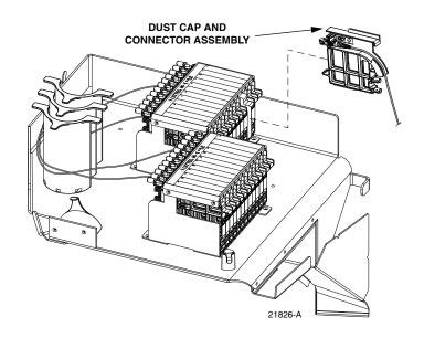
Figure 34. Inserting Dust Cap Assembly into Splitter Compartment
