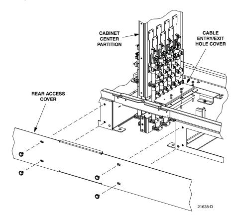
Figure 21. Cable Entry/Exit Hole Cover
