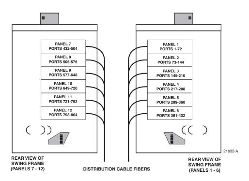
Figure 16. Distribution Cable Configuration
