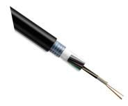
Fiber Optic Outside Plant Cable, 24-core, ECSS (Electro Chrome Coated Steel) Armored, Loose-tube, Gel-filled, 50/125 µm, OM4, Multimode, Black cable jacket
