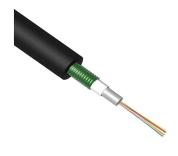
Outside Plant Fiber Optic Cable, HDPE, 8-fiber, Multimode, OM4, loose tube, gel-filled, 2000 m
