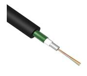
Outside Plant Fiber Optic Cable, HDPE, 12-fiber, Multimode, OM3, loose tube, gel-filled. Provides Rodent Resistance.
