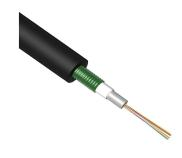
Outside Plant Fiber Optic Cable, HDPE, 24-fiber, Multimode, OM4, loose tube, gel-filled. Provides Rodent Resistance.
