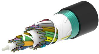
Fiber OSP cable, Single Jacket/Single Armor, 144 fiber, Gel-Free, Stranded Loose Tube, Singlemode G.652.D and G.657.A1, 200um fiber, Feet jacket marking, Black jacket color
