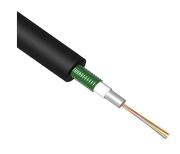
Outside Plant Fiber Optic Cable, HDPE, 12-fiber, Multimode, OM4, loose tube, gel-filled, 1000 m
