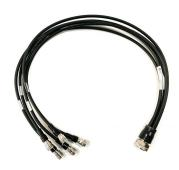
MQ Multiport cluster 5 ports cable assembly with interface type MQ female to 4.3-10 male, size 1/4", length 1.5 meters
