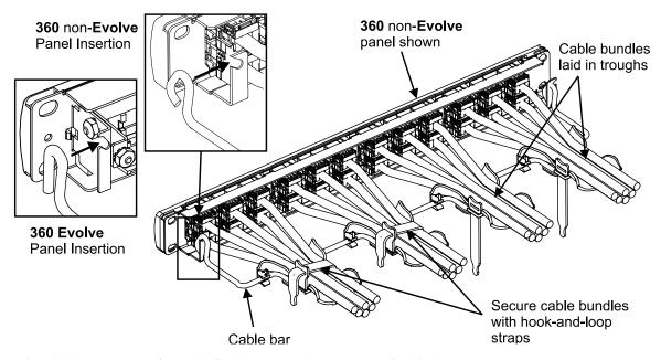
1. Attach cable bar to rear of panel. Equipment rack not shown for clarity.
