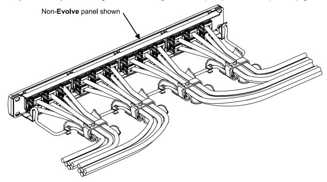
3. The figure above illustrates a typical completed installation.
