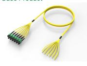
Ultra Low Loss (ULL) Singlemode G.657.A2 MPO16 (Pinned) to Unconnectorized, Fiber Trunk Cable Assembly, 192-Fiber, Dual Rated (OFNR/LSZH)
