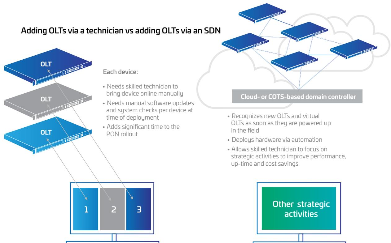
then uses automation to bring these devices online quickly and without the need for highly skilled network engineers. This hands-free onboarding makes OLT deployment a routine task and reduces the operational impact of PON rollouts.
