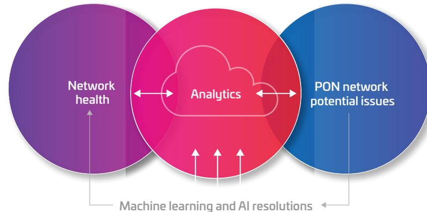
By collecting key information about the health of the network, centralizing it, and presenting it to the organizations and applications that rely on it, the service assurance platform can give PON network operators visibility into potential issues in real time. In many cases, machine learning and AI can then be employed to resolve them automatically—before they impact performance or create downtime.
