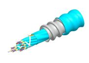
Plenum MPO Trunk Cable, interlocking aluminum armored with plenum jacket, 12 fiber
