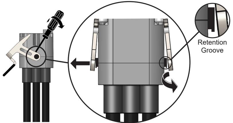
**3** Once the latch is removed, bend the two arms back to 90° so they will fit tightly back onto the housing. To reattach, latch one arm over a hinge pin then roll other arm over the housing and onto the other hinge pin.
