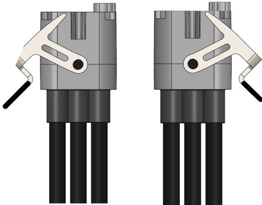
**2** Align the hole of the latch arm with the hinge pin of the connector body and pull gently away from the body, just enough to clear the end of the hinge pin. Then pull the latch arm away parallel to the body
