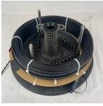
2.5 Ideally a snug fit over the rods is preferred, even if the rods lean inwards. This isn't an issue as there are rubber grommets at the base.
