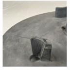
2.8 Top plate/flange – when installing the top flange, ensure the locking pin is in its parked position. Pull and turn to slide over the central column. Note the red section inside the window showing the noted pin position.
