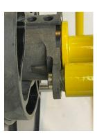
3.7 Normal usage of the dispenser is to feed the cable through the loop at the top; however, as the cable has a stop integrated on the coil to avoid the connector hitting the pulley, its preferred to feed the cable off the back of the drum to the pole.
