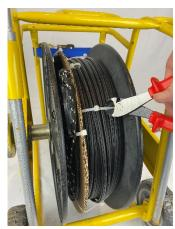
3.8 Once the cable has been pulled off, remove the sash line from the connector and the reel back on the drum for the next installation.
