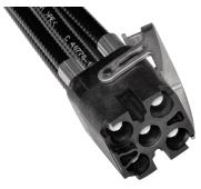
HELIAX® M-LOC Multiport cluster 5 ports SureFlex® cable assembly with interface type M-LOC latching male to NEX10 male with HELIAX® SureGuard weatherproofing, size 1/4", length 5 m
