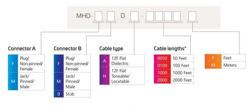
\* Cable Length shown as an example, additional cable lengths available upon request up to 2,000 ft. (600 m).
