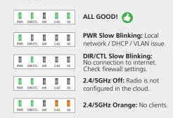
TIP #2: If the AP is advertising SSIDs, but the RUCKUS Cloud UI displays that the AP has never contacted RUCKUS Cloud, it is likely that your newly powered AP has connected to a local RUCKUS controller (SmartZone or Unleashed).
