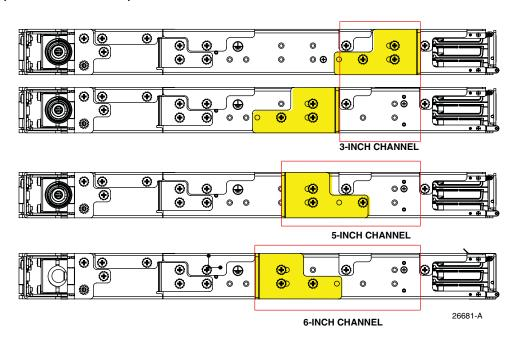
Figure 12. Mounting Positions on 3-Inch, 5-Inch, and 6-Inch Channel Racks
