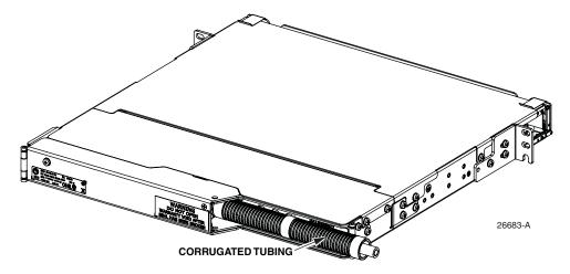
Figure 16. Corrugated Tubing on Cable
