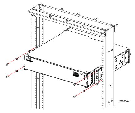
Figure 15. Securing Panel on Rack
