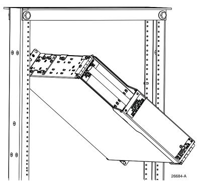
Figure 13. Rotating the Panel to Fit It on the Rack
