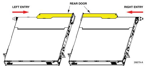
Figure 2. Left and Right Cable Entry Models
