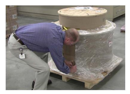
Figure 3. Cutting Off External Plastic
