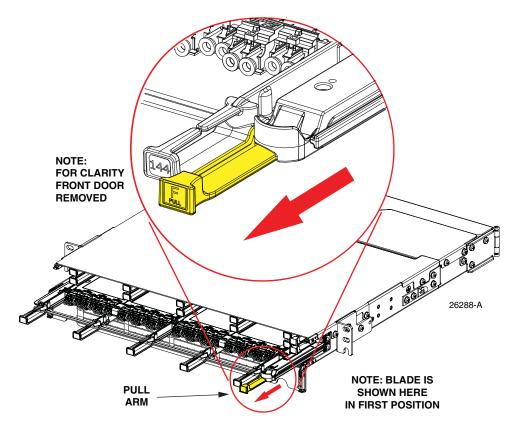
Figure 18. Sliding Out Blade to First (Access) Position
