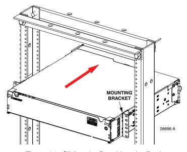
Figure 14. Sliding the Panel into the Rack
