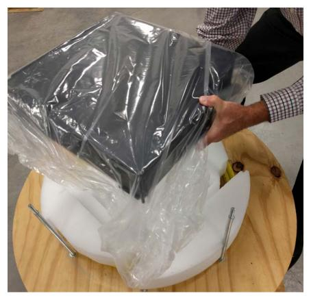
Figure 10. Removing and Unpacking Plastic Wrap
