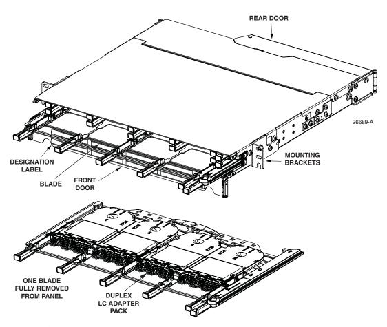
Figure 1. Main Components of SYSTIMAX EHD Pre-Terminated Panel
