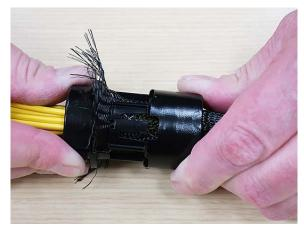
22. Snap the cap and the retainer together to capture the mesh sleeve.
