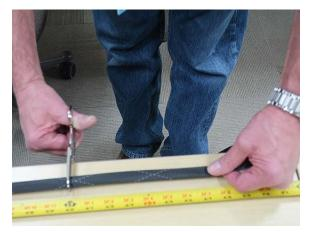
22. Tape the ends of the fiber ribbons together securely to protect them from fraying or breaking while being inserted into the mesh tubing.
