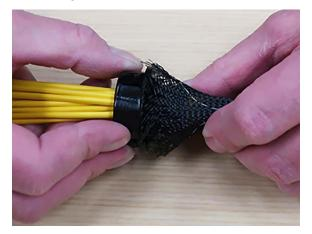
21. Slide the gland retainer toward gland cap and align the slots in the retainer with the cleats in the cap.
