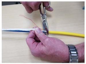
12. Carefully score the central tube near the point where it exits the cable sheath.
