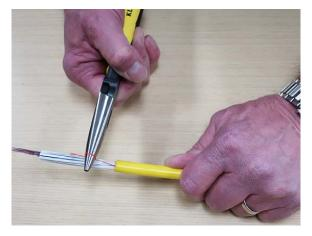
Pull the ripcord(s) to split the cable sheath back to the ring cut at the 96-inch (244 cm) mark. Needle nose pliers can be helpful to grasp and pull the ripcord(s).
