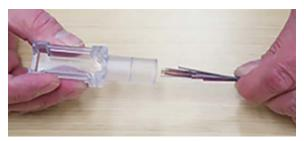
2. Slide the base up and over the cable sheath, and take note of the internal stop centered within the cylindrical base opening. For 144-fiber cable, slide the cable sheath beyond the internal stop until snug and firm. For the 288-fiber cable, slide the cable sheath up to the internal stop.
