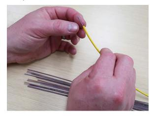
9. Slide the furcation tube all the way into the base until it meets the end of the cable.
