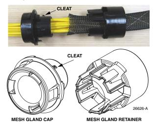
20. Anchor the mesh sleeve on the cleats on the gland cap.
