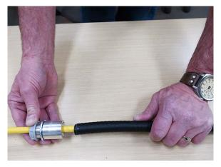
Trim back the armor jacket about 1 inch (2.5 cm) to prepare a place for the armor fitting to be threaded onto the interlocking steel armor.
