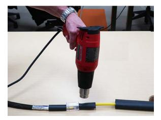
Caution! Do not allow adhesive to come in contact with skin or clothing until fully cooled. 12. After the 2.5-inch (6.4 cm) heat shrink tubing has cooled, slide the 6-inch (15.2 cm) heat shrink tubing over the fanout assembly.
