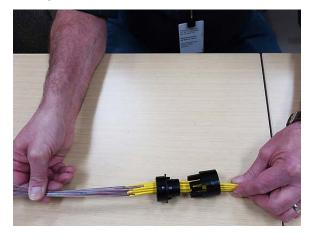
19. Slide the end of the mesh sleeve into the gland cap.
