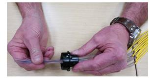
18. Slide the mesh gland cap further to the gland retainer.
