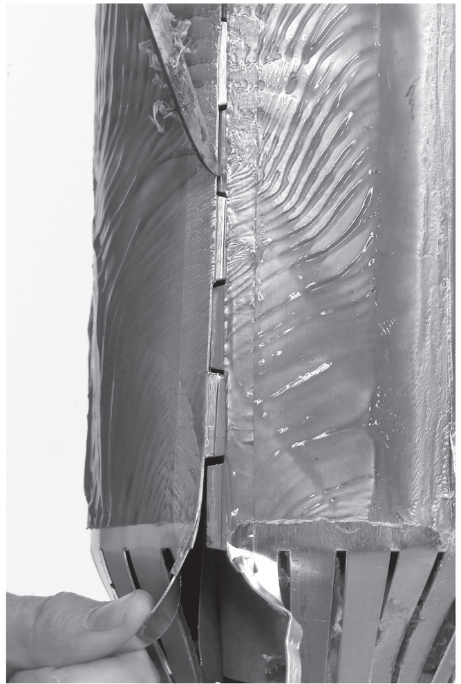
6.7 Cut the self adhering aluminum tape away from one of the canister seams and remove the canister.
