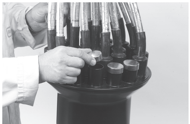
2.9 Place metal cover caps over the unused ports.
