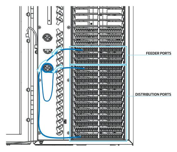
Figure 22. point to point connections
