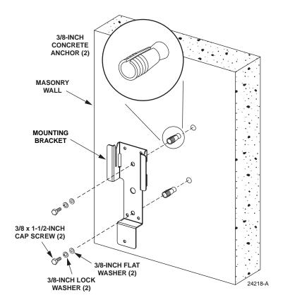
Figure 9. Installing Mounting Bracket on a Masonry Wall
