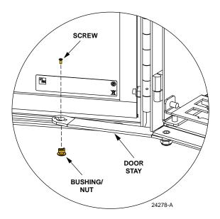
Figure 24. Door Linkage Hardware
