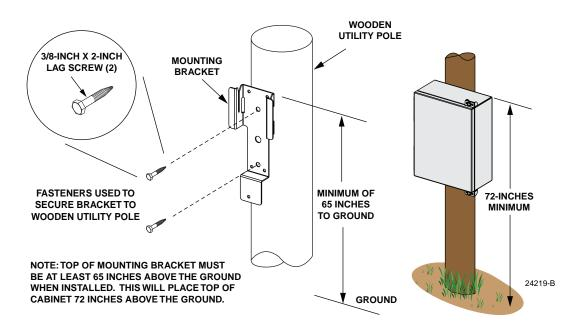
Figure 3. Installing Mounting Bracket on a Wooden Utility Pole
