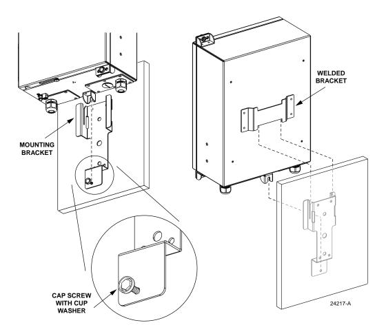
Figure 8. Installing Cabinet on Wall-Mounted Bracket
