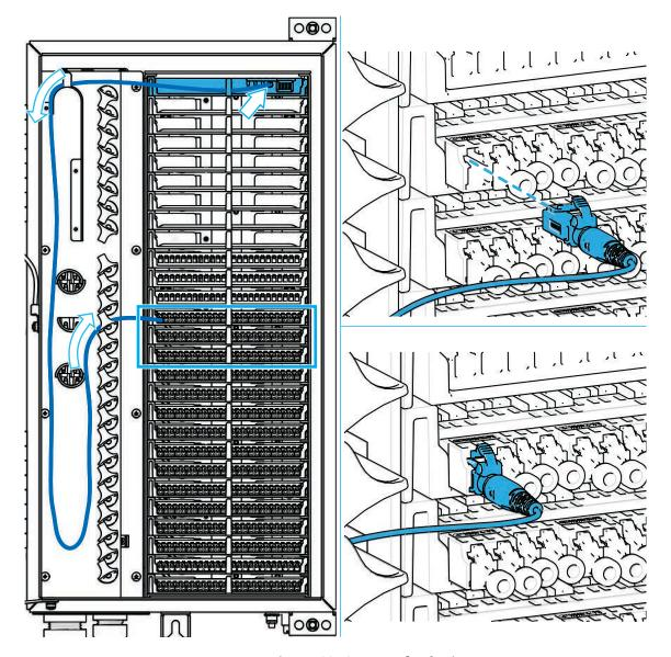
Figure 18. Connect feeder input
