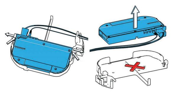
Figure 14. Remove splitter from its original tray
