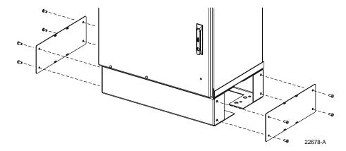
Figure 12. Removing Side Access Covers From Ground Spacer/Riser
