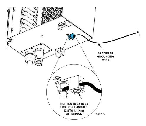
Figure 10. Grounding Wire Connection To Cabinet
