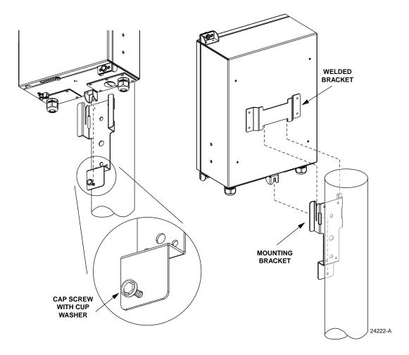
Figure 5. Installing Cabinet on Pole-Mounted Bracket
