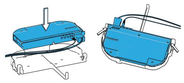
Figure 15. Install the splitter on the tray
