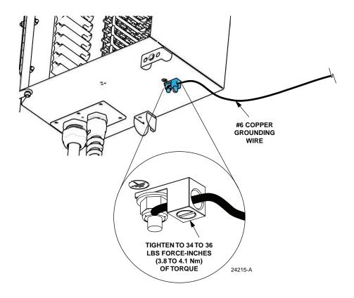
**Figure 6. Grounding Wire Connection To Cabinet**
