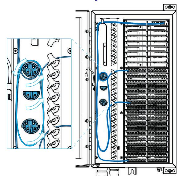
Figure 19. routing zone - drums to take up slack
