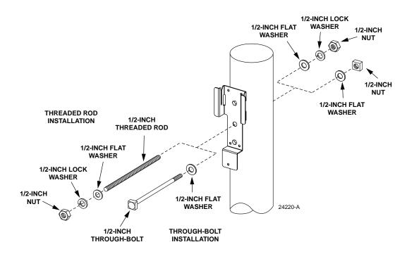
Figure 4. Threaded Rod or Through-Bolt Installation
