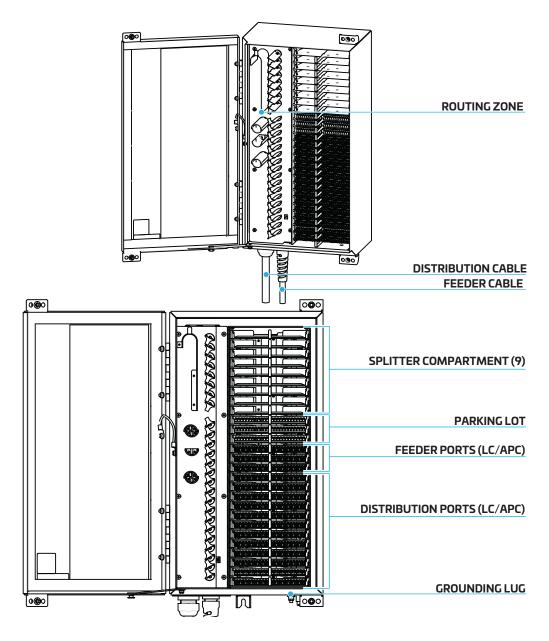
Figure 1. Splice/MPO Connector Version of the Mini 288 FDH
