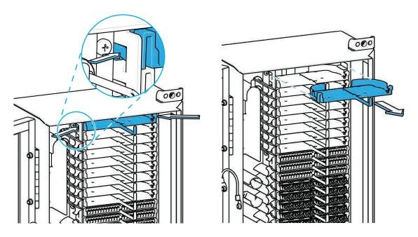
Figure 13. Remove the tray out of the slot
