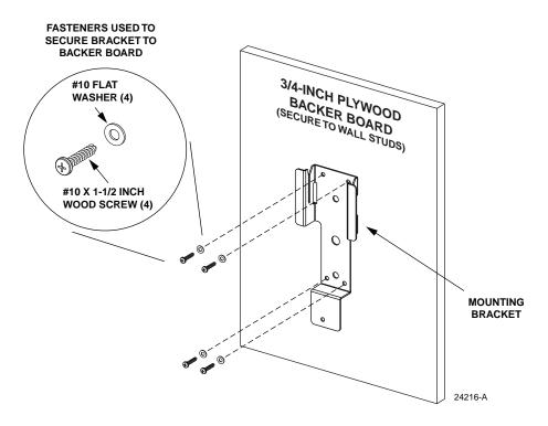
Figure 7. Securing Backer Board to Wall and Installing Mounting Bracket on Backer Board
