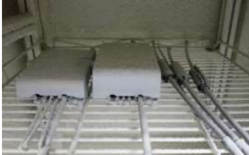
Samples in dust chamber
