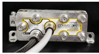
4.2.1 Once the input is connected, connect the primary RF device to Access port 1. This port provides the lowest insertion loss, -6dB. An example of a primary RF device would be an XB gateway.
