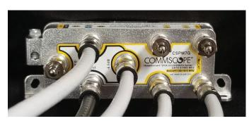
6.1.1 Once all devices have been connected, terminate all unused ports with 75-ohm RF port terminators, CommScope part # SVF59TG.
