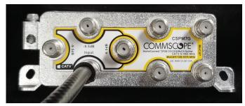
4.1.2 To activate the passive gateway, connect the input signal from the ground block and/or external drop to the RF input port.
