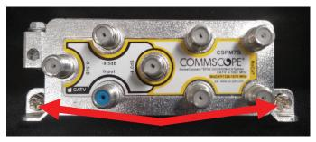
1.2.1 To mount the device with the ports facing out lay the backside of the device flush with the surface before attaching the device using the included screws and these two holes in the dual mounting tabs. This document demonstrates the installation process with the ports facing out, but the instructions are the same for both orientations.
