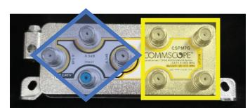
The device has two groups of four ports. One group in a diamond shape and then the other is in a square shape.
