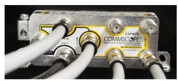
5.1.2 The MoCA ports can be utilized in any order, however for ease of installation, particularly in the APD or all ports down configuration, it is recommended to connect MoCA devices to ports 3 and 4 first.
