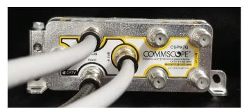
5.1.1 Now that the RF devices have been connected, The MoCA enabled devices, like X1 Terminals, may be connected to the other set of four ports.
