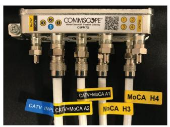
7.1.1 To attached identification labels, remove the corresponding rectangular identification label from the sheet and then wrap it around the cable sticking the two sides of the label together.
