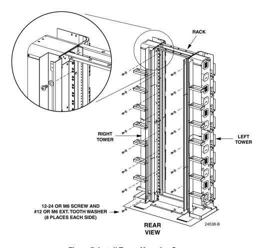
Figure 7. Install Tower Mounting Screws
