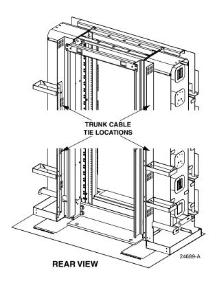
Figure 22. Trunk Cable Tie Locations
