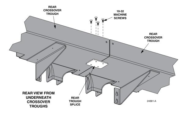
Figure 16. Rear Trough Splice Installation
