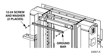
Figure 9. Optional Ground Bar Installation
