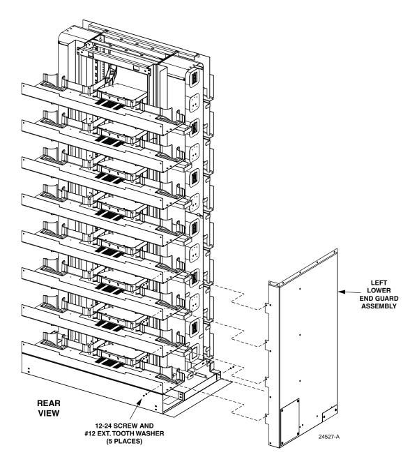
Figure 18. Lower End Guard Installation
