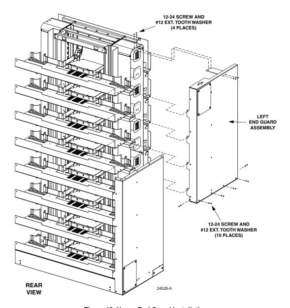
Figure 19. Upper End Guard Installation
