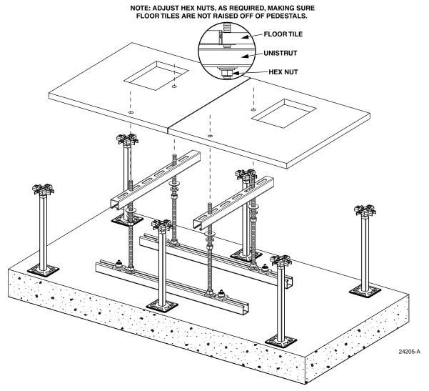
Figure 5. Typical Raised Floor Unistrut Installation
