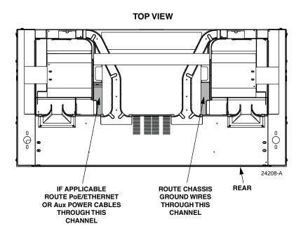
Figure 21. Ground Wire Channel
