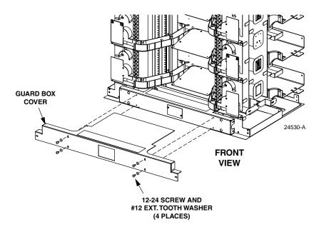
Figure 15. Installing Front Guard Box Cover
