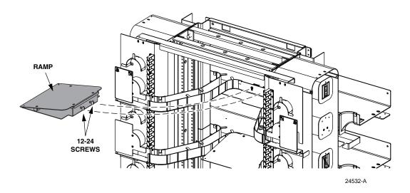
Figure 14. Install Cable Ramp
