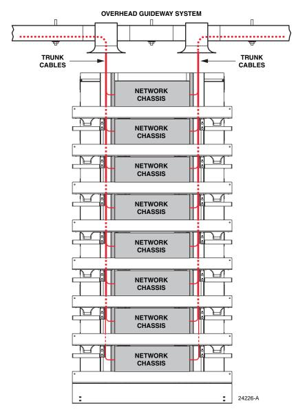
Figure 23. Overhead Trunk Cable Routing
