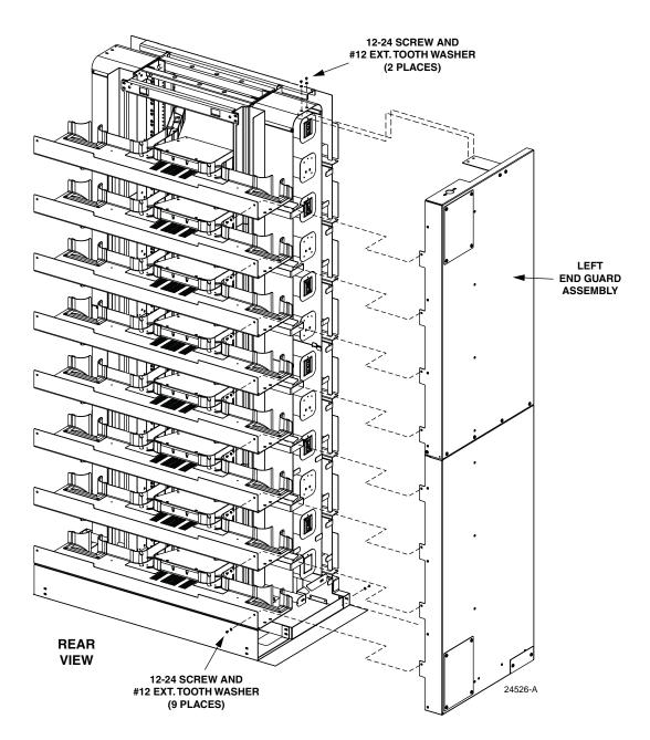
Figure 20. Mounting End Guard
