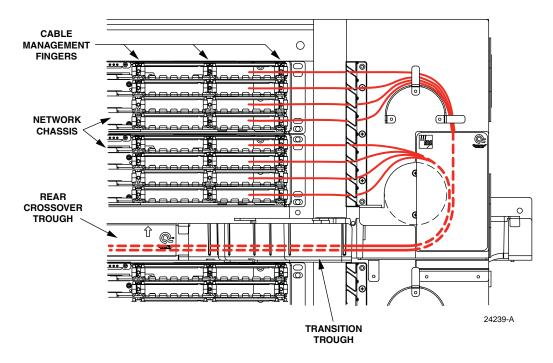
Figure 25. Cable Routing Exiting Network Chassis
