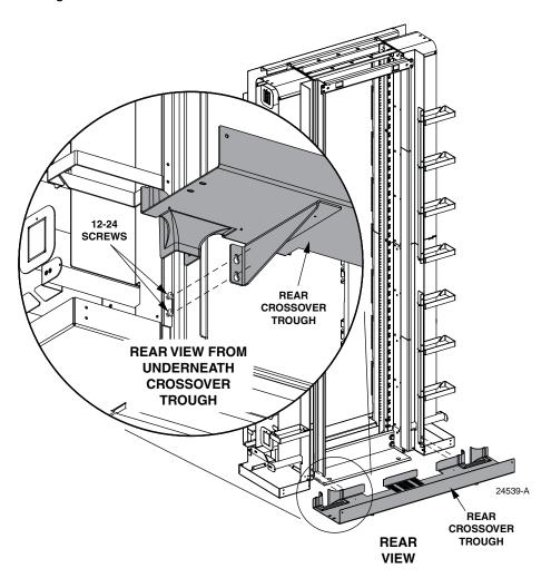
Figure 12. Rear Cable Trough
