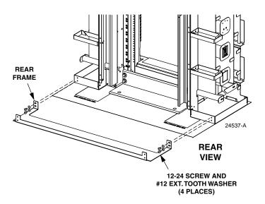
Figure 11. Installing Rear Frame
