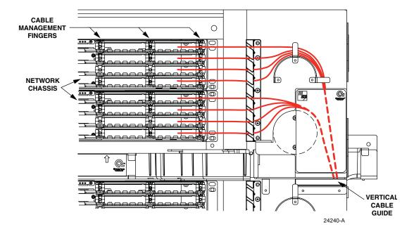
Figure 26. Cable Routing Entering Network Chassis
