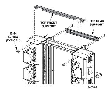
Figure 8. Install Top Front and Rear Supports
