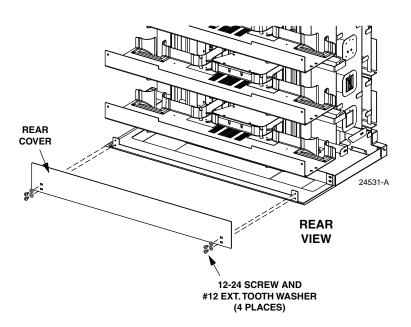
Figure 17. Installing Rear Cover
