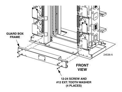
Figure 10. Installing Front Guard Box Frame
