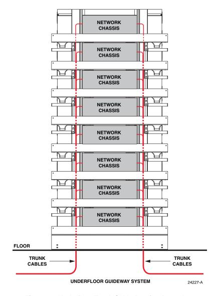
Figure 24. Underfloor Trunk Cable Routing Procedure
