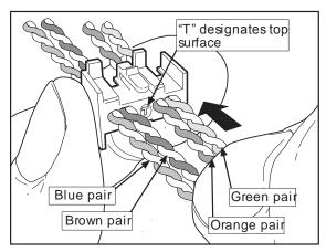
Figure 2. Feed Pairs into Termination Manager
