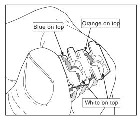
Figure 3. Fold Pairs Back into Slots
