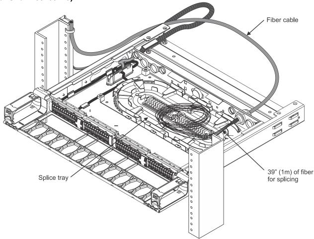
**Note**: Stackable splice tray kit (760148502) is ordered separately from shelf. Refer to instructions enclosed with that kit for all details not covered here. Each splice tray will accommodate up to 48 fusion splices. If more splice capacity is required, an additional splice tray may be stacked and attached to the first for a total of 96 splices.
