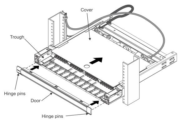
Install top cover and trough door (both provided) to shield shelf from foreign particles. The cover, which is made of clear, flame-retardant plastic, slides on and off shelf. The door for the patch cord trough is hinged and has touch-latches for closing and opening.
