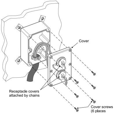
1. Secure cover to front of box with the six screws provided.
