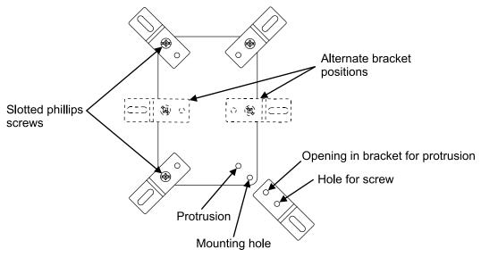
1. Install offset brackets on rear of box, diagonally from the corners, using slotted phillips screws provided. Raised protrusions molded into rear of box are used to properly align mounting brackets.
