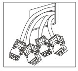
Feed wires through the frame, in between the two latch bars as shown.
