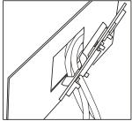
Install frame in cutout by hooking lower latch bar over the bottom edge of the panel cutout.
