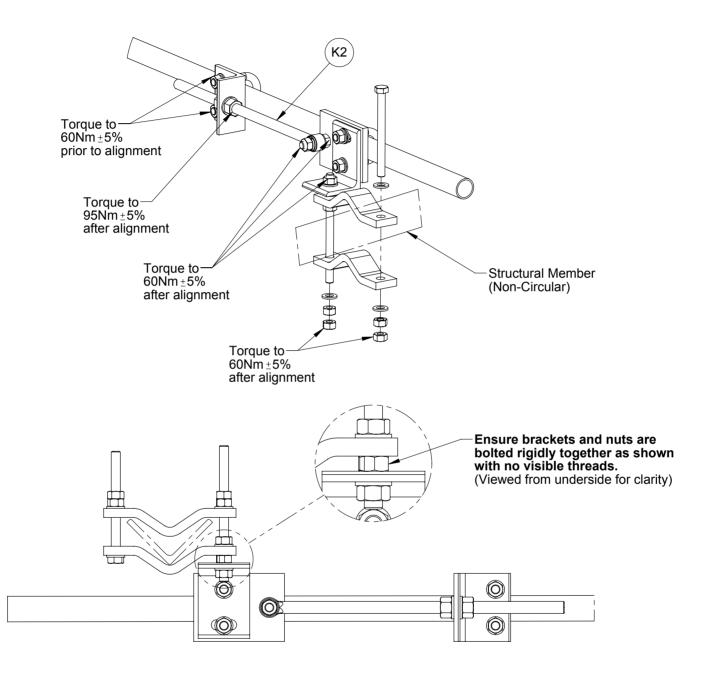
Clamps must be attached to a non-circular structural member capable of supporting 6187N in accordance with TIA-222.
