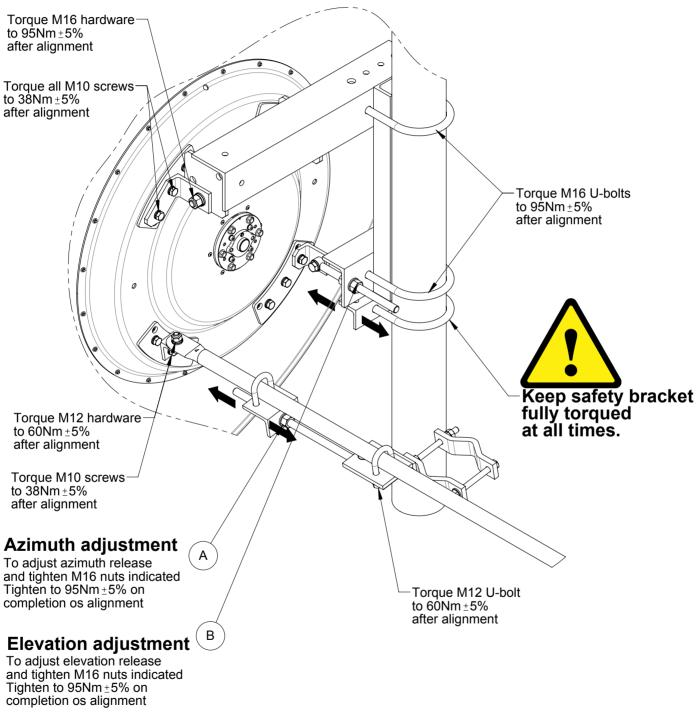
Ensure all hardware is tightened to specified torque after completion of azimuth and elevation alignment
