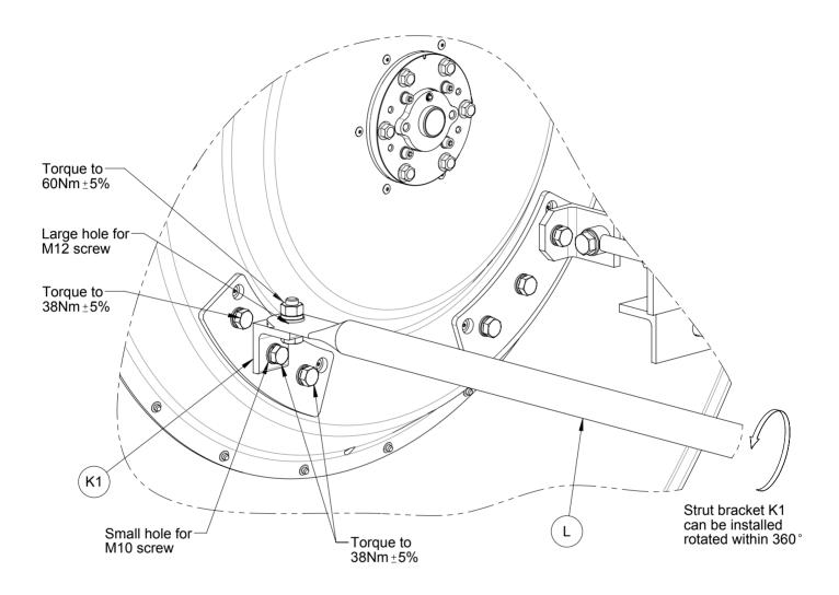
Strut to be loosely fitted until alignment is complete then tighten all fixings to torque specified.
