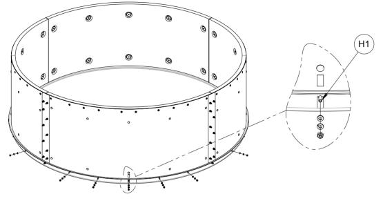
Fit bolts, washers, lock washers and nuts to remaining holes of assembly and tighten.
