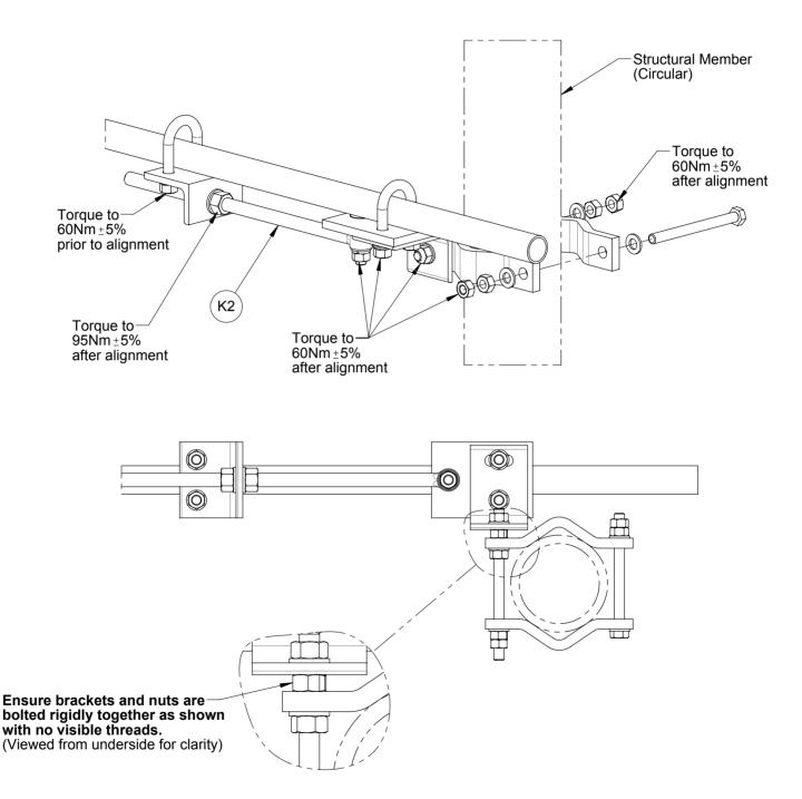
Clamps must be attached to a circular structural member (Dia 48mm - 120mm) capable of supporting 6187N in accordance with TIA-222.
