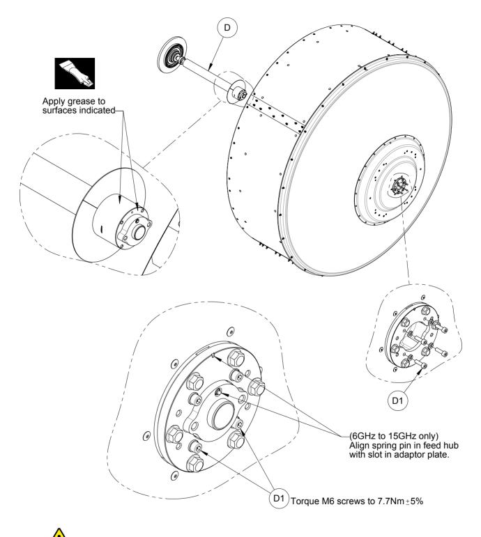
After assembly, remove excess grease from internal reflector surface.
