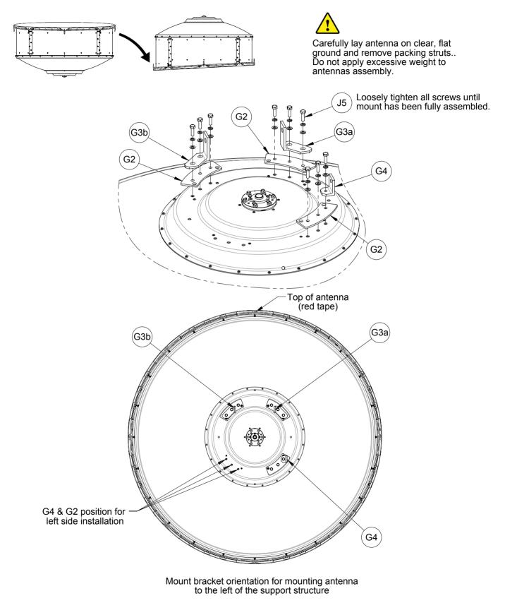
For mounting the antenna to the right of the supporting structure assemble bracket G4 along with associated plate G2 in position indicated.
