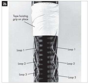
3 Fold the lace in half to form a crease at the center. Starting at the top, pass the lace through the first loop pair so that the crease is between them as shown in Figure 3a. Cross the lace ends and pass them through the second loop pair from the underside and pull at right angles in the same way as lacing a shoe (see Figure 3b).
