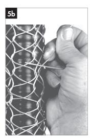
6 IMPORTANT: First, remove the tape from the tip of the hoisting grip. Then, place both hands firmly around the bottom of the grip and slide them upward to the top as shown in Figure 6. This pulling action removes slack throughout the grip. Repeat this twice.
