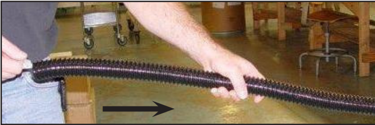
Access front section of the clear poly tube from the protection tube. While holding the clear tube, gently push the protection tube toward cable. Make sure protection tube is straight while pushing.
