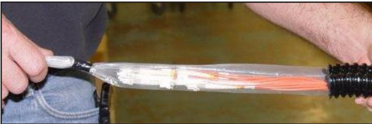
Expose just enough clear tube outside the protection tube for access all optical connectors.
