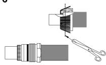
7 Remove 5.0 mm (0.197") of foam. Remove all foam/glue residue from the center conductor.
