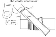
Chamfer the center conductor at a 45° angle.
