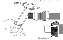
Cut off the redundant braid as shown.
