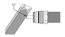
The cable center conductor must be straignt and aligned with the connector inner 9 contact. Insert the cable into the connector body until stopped; the center conductor must be inserted into the connector inner contact fingers. Tighten the connection to the torque value of 8.8-10.8 N.m.
