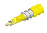
Fiber indoor cable, TeraSPEED® Plenum MPO Trunk, interlocking aluminum armored with plenum jacket, 288 fiber multi-unit with 12 fiber subunits, Singlemode G.652.D and G.657.A1, Feet jacket marking, Yellow jacket color
