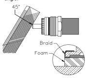
The cable attachment must be straight and aligned with the hole of connector inner contact. Insert cable attachment into connector body until stopped; the center conductor must be inserted into the connector inner contact fingers. Tighten the connection to the torque value of 44-53 lb-in (5.0-6.0 Nm). Note: Do not turn connector body, turn clamp nut attachment.
