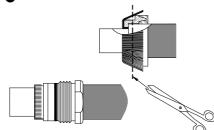
Remove 5.0 mm (0.197") of foam. Remove all foam/glue residue from the center conductor.
