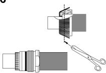
Remove 8.5 mm (0.335") of foam. Remove all foam/glue residue from the center conductor.
