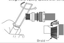
Cut off the redundant braid as shown.
