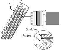
The cable attachment must be straight and aligned with the hole of connector inner contact. Insert the cable attachment into the connector body until stopped; the center conductor must be inserted into the connector inner contact fingers. Tighten the connection to the torque value of 60-80 lb-in (6.8-9.0 Nm). Note: Do not turn connector body, turn cable attachment.
