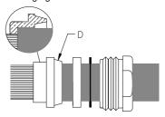
Fold braid around part D and comb braid as shown, the braid should be straight and equally spaced after comb.
