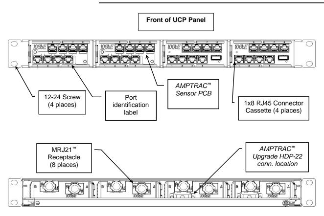
Figure 1 (1-1671594-1 panel with AMPTRAC Cassette 2153091-1 and Standard Cassette 2153115-1 as shown. Use appropriate customer drawing for other panel views)
