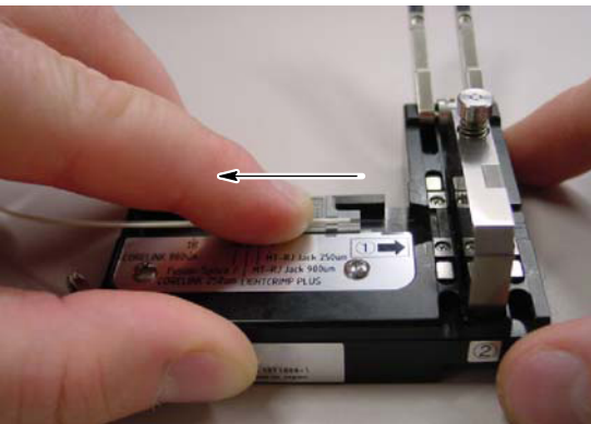
11. Move the fiber slide back.
