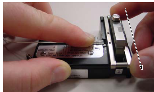
9. Slide the carriage forward (in the direction shown).
