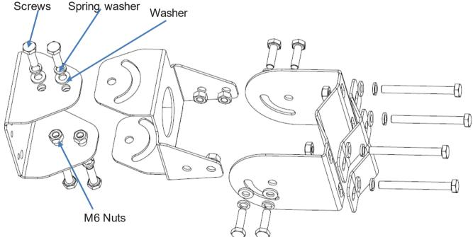
Fit these seven parts above together and fasten them with screws M6, nuts M6, spring washers, and washers.
