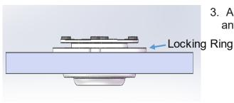
3. Adjust the locking ring to fasten the antenna mount to the ceiling.
