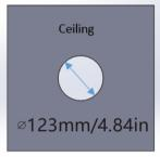
1. Cut a hole with a diameter of Ø123mm/4.84in into the ceiling where the antenna is supposed to be installed.
