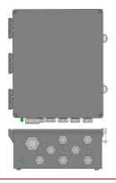
Hybrid Junction box, Fiber and power cable connection enclosure. Manages one 4-core or 8-core power trunk 12 AWG up to 6 AWG, one 24 fiber trunk cable and up to 6 hybrid tails. Internal trunk grounding. IP67
