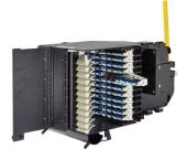
Next Generation Frame (NGF) Fiber Termination Block with IFC Cable, Dual Rated, Rollable Ribbon singlemode 200u, 288 LC/UPC to Stub tail, left oriented, upward cable exit, black
