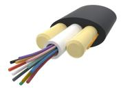
Fiber outdoor drop cable, LightScope ZWP® Self-Supporting All-Dielectric, Singlemode G.652.D and G.657.A1, 4 fiber Arid Core construction, Gel-filled, central loose tube, Meter jacket marking, Black jacket color
