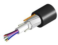
Fiber indoor/outdoor drop cable, LightScope ZWP® All-Dielectric, Singlemode G.652.D and G.657.Al, 12 fiber Arid Core construction, low smoke zero halogen (LSZH), Gel-filled, central loose tube, Feet jacket marking, Black jacket color, Dca flame rating
