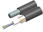
Fiber outdoor drop cable, LightScope ZWP® Self-Supporting Non-Armored Figure-8, Singlemode G.652.D and G.657.A1, 6 fiber Arid Core construction with 0.109 in messenger, Gel-filled, central loose tube, Feet jacket marking, Black jacket color
