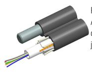
Fiber outdoor drop cable, LightScope ZWP® Self-Supporting Non-Armored Figure-8e, Singlemode G.652.D and G.657.A1, 4 fiber Arid Core construction with 0.109 in messenger, Gel-filled, central loose tube, Feet jacket marking, Black jacket color
