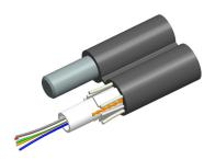
Fiber drop cable, LightScope ZWP® Self-Supporting Non-Armored Figure-8, Singlemode G.652.D and G.657.A1, 1–fiber Arid Core construction with 0.109 in messenger, Gel-filled, central loose tube, Feet jacket marking, Black jacket color
