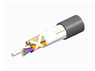
Fiber indoor/outdoor cable, LightScope ZWP®, Single Jacket All-Dielectric, Plenum Rated, Gel-Free, Singlemode G.652.D and G.657.Al, 36 fiber, Stranded Loose Tube, PVDF jacket, Feet jacket marking, Black jacket color
